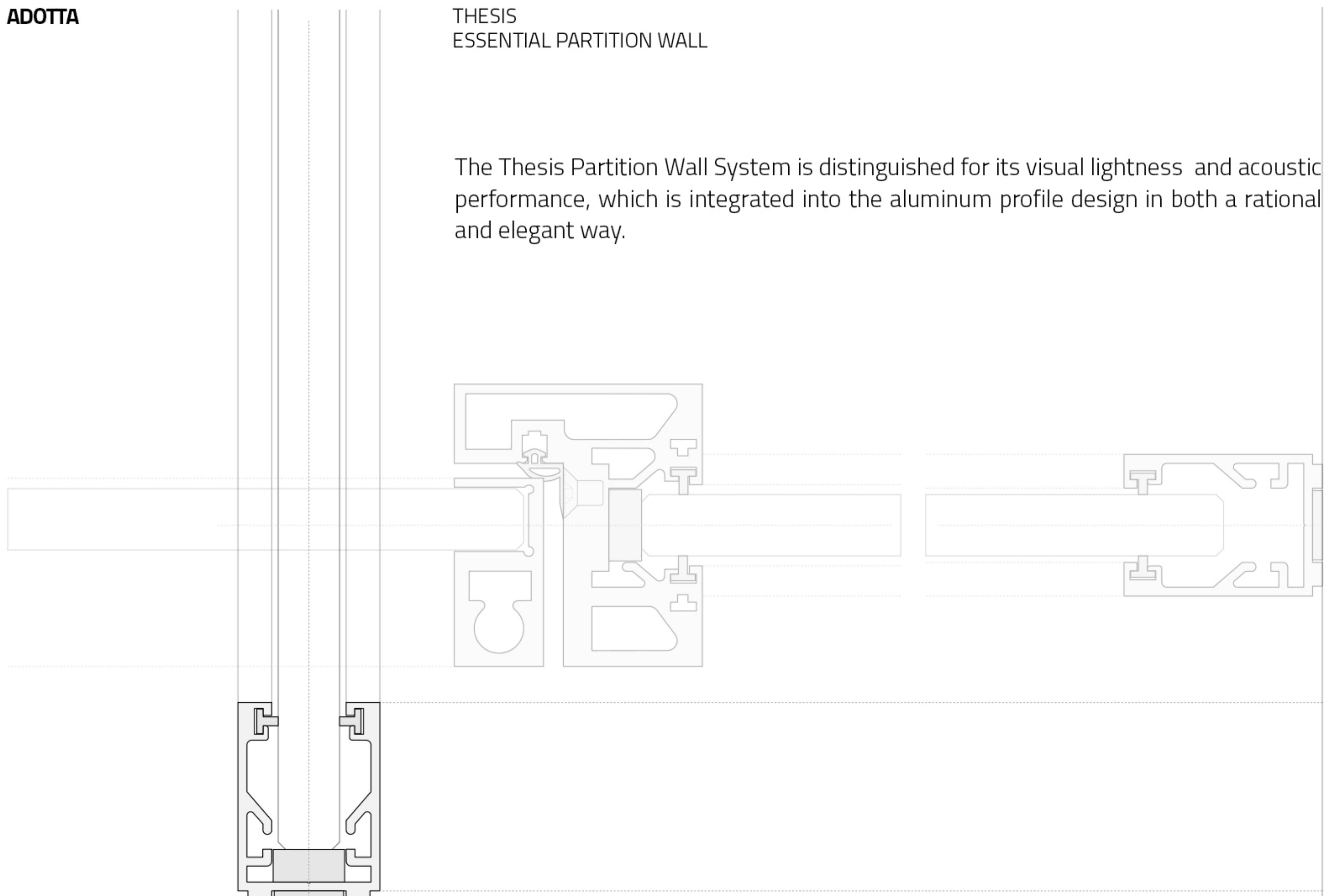
Thesis is built with 40 mm extruded aluminum profiles that can hold tempered or laminated glass panels of 12 mm thicknesses.
