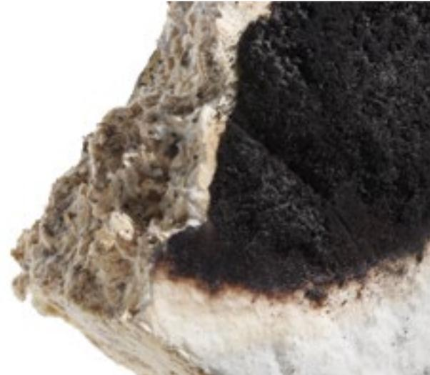
Mogu Acoustic panels are naturally fire retardant thanks to the ability of mycelium to slow down flame spread and form char. Even without treatment, Mogu Acoustic panels carbonize and burn very slowly. Thanks to an eco-friendly treatment, their fire reaction is further improved to class B-s2-d0, which allows their application in every public space.
